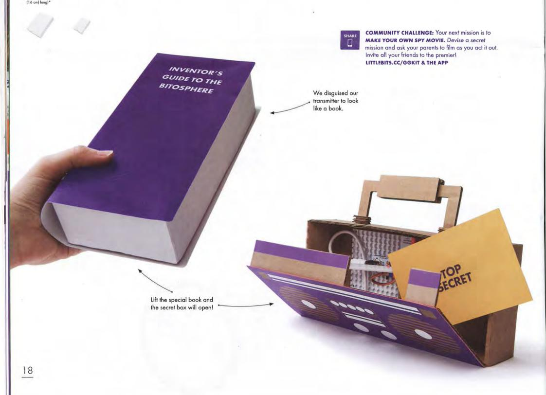
BUILD A TRIGGER BOX and place your transmitter circuit within it. Cut out a small hole, and use Glue Dots to stick the light sensor and wireless transmitter to the side with the hole. The light sensor should be facing out of the hole. Exposing the light sensor will activate the wireless interaction.
